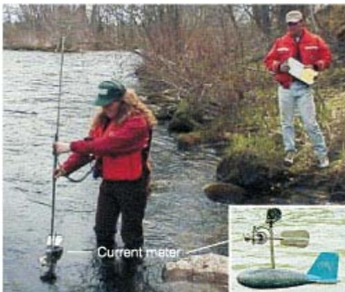
Amy Wehnke, USGS hydrologic technician, wades into a stream to measure streamflow using a current meter. Sandy Ward, USGS hydrologic technician standing on the shore, records the streamflow data Amy is measuring.
